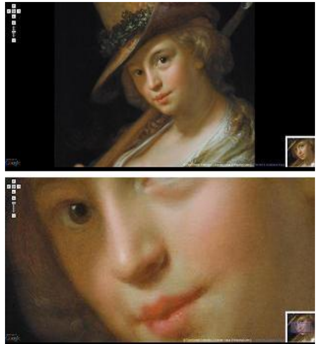
Fig. 3. Low resolution version of the whole image (above); when zooming in, higher resolution sections are transferred (below).
