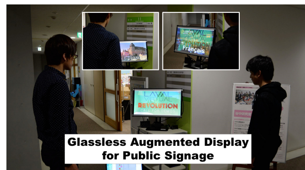
Figure 1: Prototype of proposing Glassless Augmented Display for public signage. Each viewer can see different images and audios from different directions.
