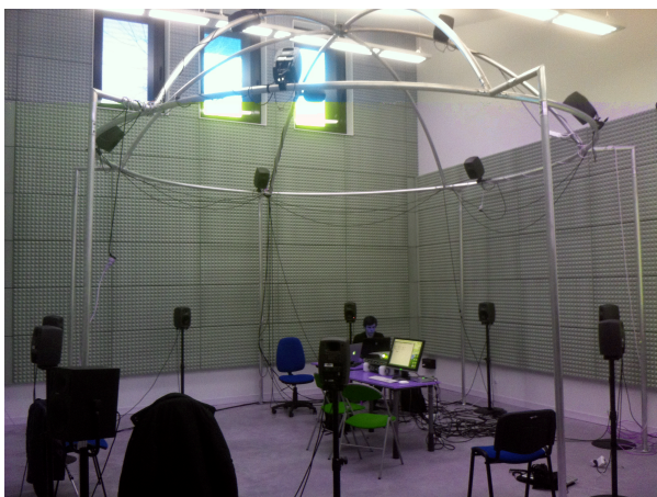
Figure 11. CICM's HOA 16 channels semi dome.
