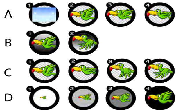
Figure 4: Lenticular lens effects. A: 3D, B: Flip, C: Animation, D: Morph
